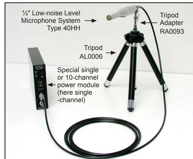
Fig. 2 A complete single-channel low-noise level measuring system
