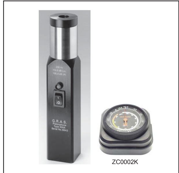
Fig. 1 Pistonphone Type 42AA 114 dB at 250 Hz. Shown with Barometer ZC0002K - for applying corrections for ambient pressure
