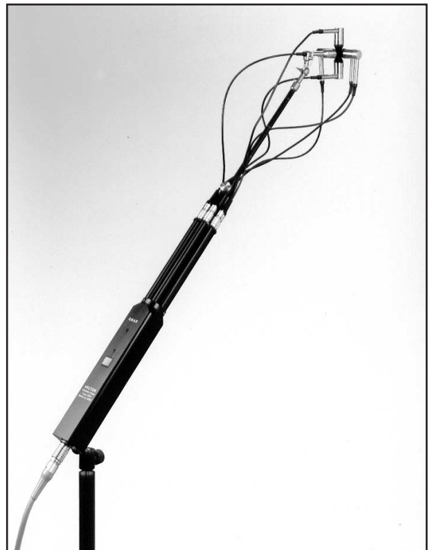
Fig. 1 Vector Intensity Probe Type 50VI version 1 for 3-dimensional sound-intensity measurements
