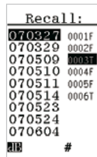
All measurements are stored using the actual date as current directory name
