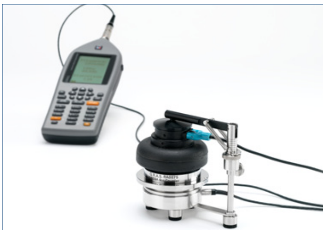
TDH-39 Supra-aural earphones mounted on the NBS 9-A / IEC 60318-3 6cc Coupler. This setup is based on a 1" measurement microphone.
