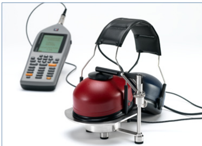
HDA-200 Circum-aural earphones mounted on the IEC 60318-2 Ear Simulator (high-frequency coupler). This setup is based on a 1/2" measurement microphone.
