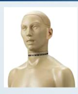
Improved materials KEMAR's previous fiber glass construction has been updated to a composite plastic construction that is more rugged and user friendly.
