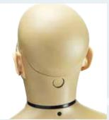
The scalp is easily removed with the new release button which provides easy access to the inside of KFMAR.
