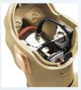
ear simulators Mount and dismantle the ear simulators with one hand for ear-canal exchange or calibration.
