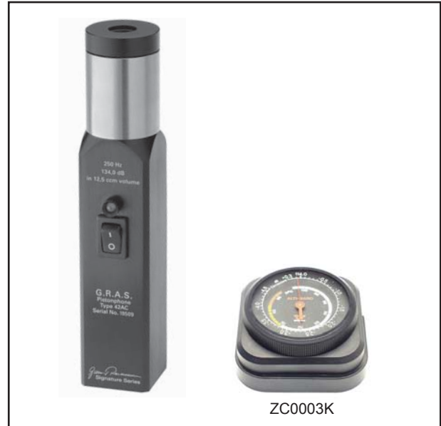
Fig. 1 Pistonphone Type 42AC: 134 dB at 250 Hz. Shown here with Barometer ZC0003K, which is used for applying corrections for ambient pressure
