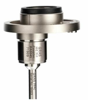
Connection: 200 V/LEMO Volume: Complex Dyn range: 26 dB(A) to 164 dB ANSI: S3.7 The GRAS 43AE Ear Simulator Kit according to ITU-T Rec. P57 Type 3.2 is for acoustically testing supra-aural earphones, telephone handsets and loudspeakers, and complies with the international requirements: ITU-T Recommendation P.57 (08/96) "Serie P: Telephone Transmission quality. Objective measuring apparatus: Artificial ears".
