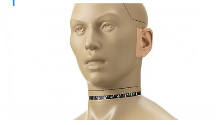
Connection: 0 V/CCP or 200 V/LEM0 Channel(s): 2 ANSI: S3.36, S3.25 IEC: 60318-7 The 45BB KEMAR head and torso is a configurable acoustic research tool that simulates the changes that occur to sound waves as they pass a human head and torso. Its equivalent with mouth simulator is <u>GRAS 45BC</u> <u>KEMAR Head & Torso, non-configured</u>
