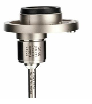
Connection: 0 V/CCP Volume: Complex Dyn range: 25 dB(A) to 150 dB ANSI: S3.7 The GRAS 43AE-S1 Ear Simulator according to ITU-T Rec. P57 Type 3.2, Prepolarized is for acoustically testing supra-aural earphones, telephone handsets and loudspeakers, and complies with the international requirements: ITU-T Recommendation P.57 (08/96) "Serie P: Telephone Transmission quality. Objective measuring apparatus: Artificial ears".
