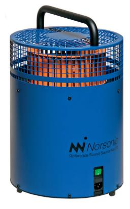
The reference sound source Nor278 is designed to produce a stable and uniform sound power output with unique long-term stability. The high sound power output makes it ideal for sound power measurements in a noisy environment. The rugged, but yet portable and light weight construction is perfect for field us as well a laboratory use.
