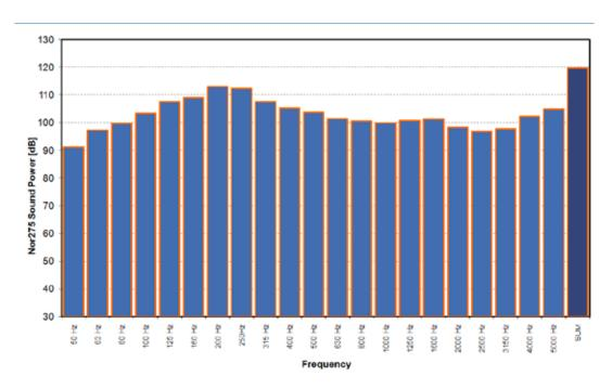
Typical sound power level vs. frequency of the Hemi-dodecahedron Loudspeaker Nor275 when used with the pink noise source and equalizer included in the Power Amplifier Nor280.
