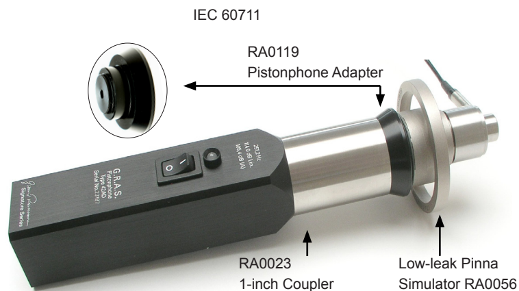
Fig. 3.5 Calibration-check set-up. Make sure that the rubber seal of the Pinna Simulator seats firmly inside the Pistonphone Adapter
