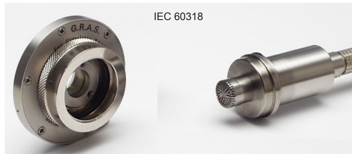
Fig. 3.3 Showing the two halves of the snap coupling to give quick access to the microphone
