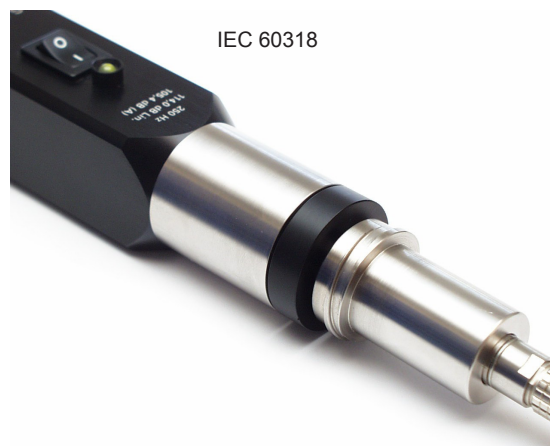
Fig. 3.4 Gently push the microphone into the Pistonphone's coupler until it reaches the stop
