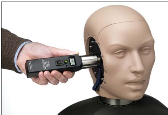
Fig. 19. Place the pistonphone onto the ear canal.
