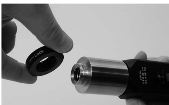
Fig. 17. Loosen the retention collar on the pistonphone.
