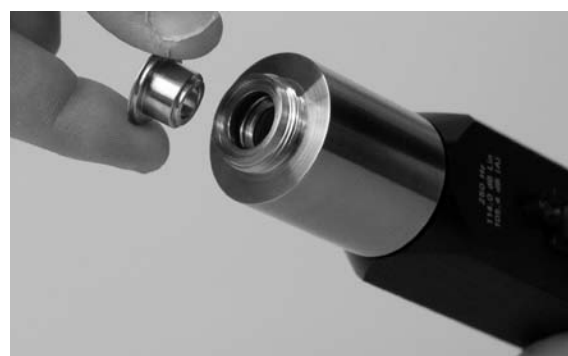
Fig. 18. Mount the adapter RA0157 on the pistonphone.
