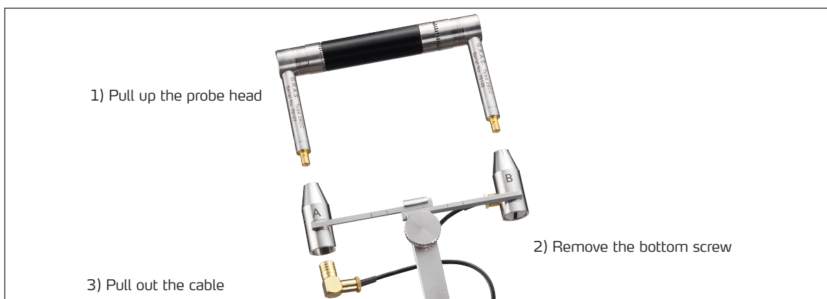
Fig. 8. Releasing the cable connectors from the holder assembly
