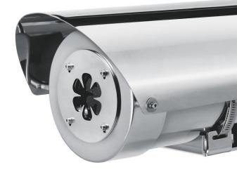
**Workswell SAFETIS EX-proof** camera offers great resolution of 640 x 512 px, sensitivity of 50 mK (0.05 °C) and fast response within milliseconds. The powerful communication interface allows connecting SAFETIS camera directly to any computer via Web-server or directly to **SAFETIS Control Unit** via Ethernet RJ45. The SAFETIS camera has integrated 7 digital outputs in the camera and 7 digital outputs in **SAFETIS Control Unit** that can be triggered at the same time if needed.
